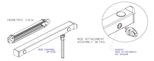
Please note that if the rod attachment is removed it cannot be reinserted.
