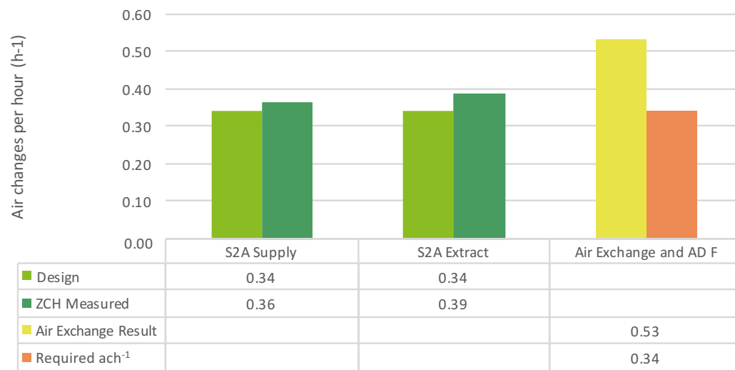
Chart 2c: Site 2 Plot A: MVHR Air Flow and Air Exchange Measurements
